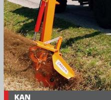
KAN is a ditch cleaner, designed for cleaning and profiling ditches along roads.
