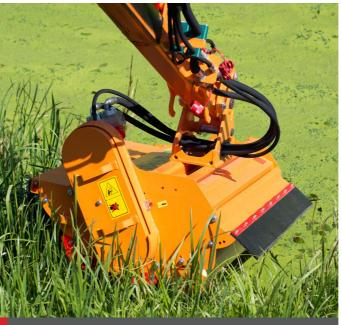
HYDRA is a combined working head for mowing and cutting vegetation up to 50 mm thick. Efficient operation of the HYDRA mowing head is enabled by the design of its key parts. The spiral distribution of the blades reduces energy consumption, and the increased opening at the back of the head allows a high flow of material, and accordingly, a higher mowing speed.
