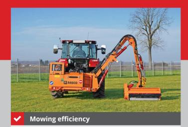
The advanced intuitive control system ensures easy operation of the arms and working tools, while the external oil cooler located next to the hydraulic power unit prevents the oil from overheating and ensures long-lasting and uninterrupted mowing.
