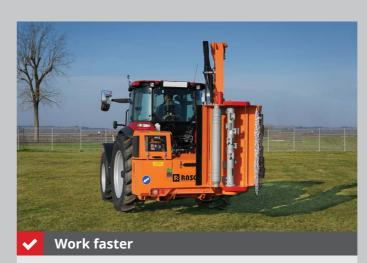
The NEVA rear boom mower can be quickly mounted and dismounted on/off the tractor rear three-point hitch, which equips the tractor for the mowing season, or free it for other purposes. Working tools can also be changed quick and easy, turning the mower into a tool for cutting branches or ditch cleaning.
