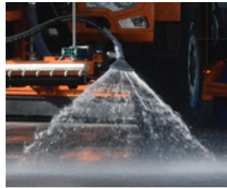
High flow lateral nozzles can be mounted on the left and right ends of the ramp and directed individually via the hydraulic system
