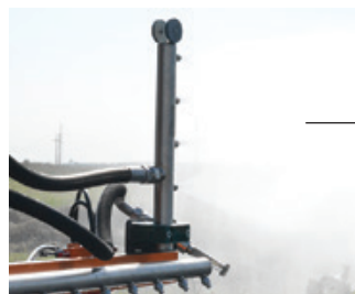
The side vertical ramp allows the washing of guardrails located along the edge of the road
