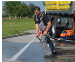
A manual high-pressure washer helps washing hard-to-reach objects
