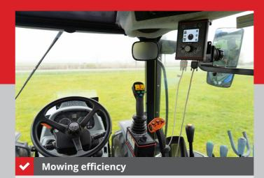
Advanced intuitive control system enables simple operation of the arms and the working tool, while the external oil cooler next to the aggregate prevents overheating of the oil, ensuring long-lasting and uninterrupted mowing.
