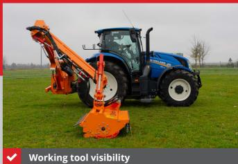
Specially designed arm kinematics bring the working tool in the user's visual field, increasing the mowing visibility and the safety of operation.
