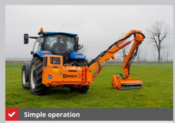
SPECTRA rear boom mower is simple to mount and demount from the rear three-point attachment, quickly equipping the tractor for the mowing season as well as quickly freeing it for other purposes.
