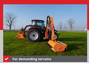
Robustness and arm reach of up to 5, 6 or 7 meters guarantee efficient maintenance of canals along open roads or embankments along waterways. The choice between three different versions of the hydraulic power unit allows complete adjustment to the terrain.
