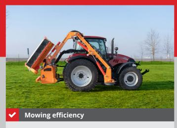
The BRK is installed laterally, between the front and rear axles of the tractor, which makes it stable and safe. The operator has excellent working visibility, more comfort, and can easily avoid obstacles (traffic signs, etc).
