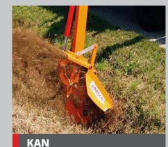
KAN is a ditch cleaner, designed for cleaning and profiling ditches along roads.
