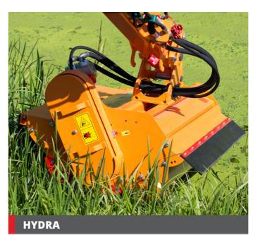
HYDRA is a combined working head for mowing and cutting vegetation up to 50 mm thick. Efficient operation of the HYDRA mowing head is enabled by the design of its key parts. The spiral distribution of the blades reduces energy consumption, and the increased opening at the back of the head allows a high flow of material, and accordingly, a higher mowing speed.
