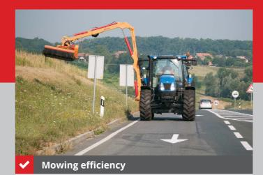
The BRKT is installed laterally, between the front and rear axles of the tractor, which makes it stable and safe. The operator has excellent working visibility, more comfort, and can easily avoid obstacles (traffic signs, etc).
