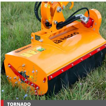
TORNADO mowing heads are an ideal choice for maintaining smaller vegetation. They are designed to provide the possibility of using two types of blades for cutting vegetation of different thickness, with a diameter of 15 to 30 mm.
