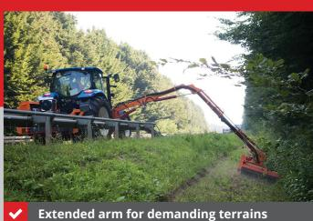
The working reach of up to 8 meters, enabled by a telescopic
