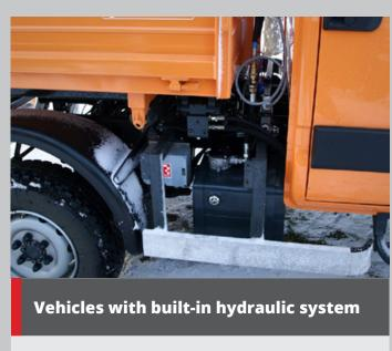
JUNIOR spreaders can be powered using a built- in hydraulic system of the vehicle if it is designed according to the EN ISO 15431 standard.
