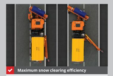
For maximum efficiency of clearing snow on motorways, we recommend that KALNIK XL is used in combination with the BSP side plough in an echelon ploughing configuration.
