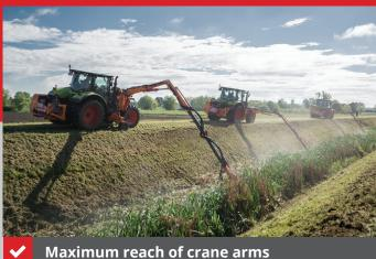
MAXIMA is available in 8, 9 or 10 meter crane arm configurations. A large reach is provided by telescopic arms made of special-purpose steel that can easily withstand the increased strain of the arms when mowing.
