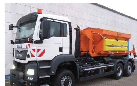
Mounting on vehicles equipped with a hooklift system
