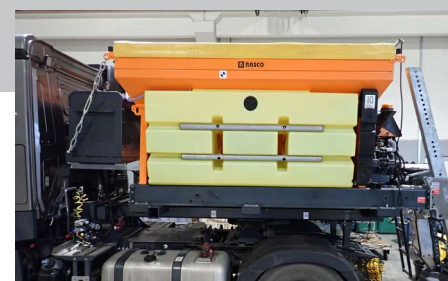
Mounting on the saddle of the vehicle
