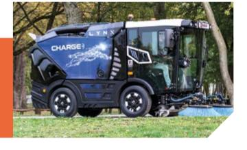
Both sweepers have a water recirculation system, ensuring a smooth flow of collected material and additional dust suppression. This feature plays a crucial role in saving fresh water, contributing to the sustainable operation of the sweeper. The sweepers are designed to suppress dust (PM 10/2.5 certified), contributing to better air quality.
