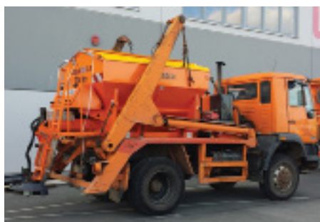
Mounting on container lifting system
