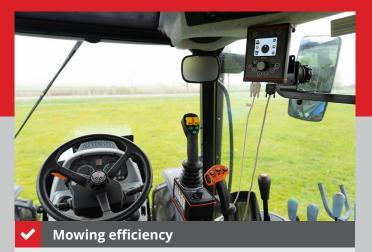
Advanced intuitive control system enables simple operation of the crane arms and the working tool, while the external oil cooler next to the aggregate prevents overheating of the oil, ensuring long-lasting and uninterrupted mowing.
