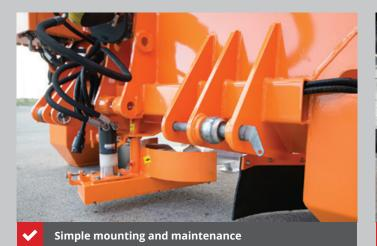
The spreader is mounted on the rear tractor three-point attachment, and powered via the self-loading system.
