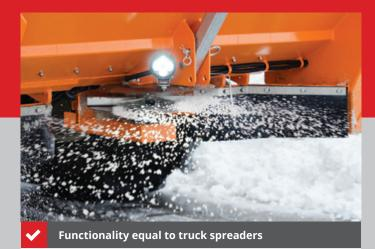
The asymmetry and width of spreading, as well as the quantity of spreading material are controlled from the cabin of the tractor with an EPOS control unit without the need to look away from the road, which makes TRP equal to truck spreaders with regard to functionality and precision of spreading.
