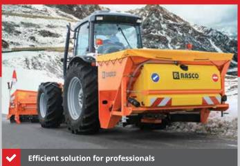
The TRP spreader turns every tractor into a winter road maintenance vehicle. Its 0.4 to 1.5 m³ dry agent capacity and 500 L liquid agent capacity make TRP a good choice for urban and rural areas where simplicity, efficiency and value for money are the key factors for the selection of road maintenance equipment.
